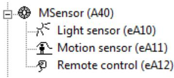
DALI MSensor 02 consists internally of three device classes, which are listed individually in the DALI device tree diagram:
