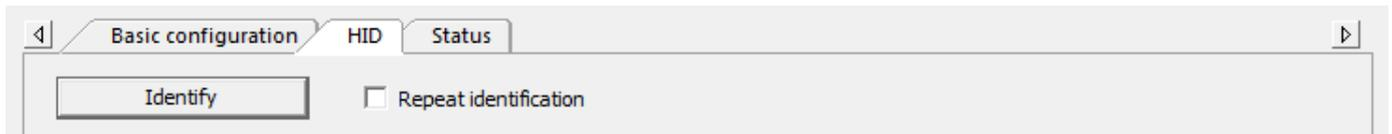
Here you can directly display the address of the high-pressure discharge lamps via the status LED on the device. For this purpose, the address is converted into a six-digit binary number, which is represented as a flashing pattern. The red LED stands for binary number 0, the green LED for binary number 1.
