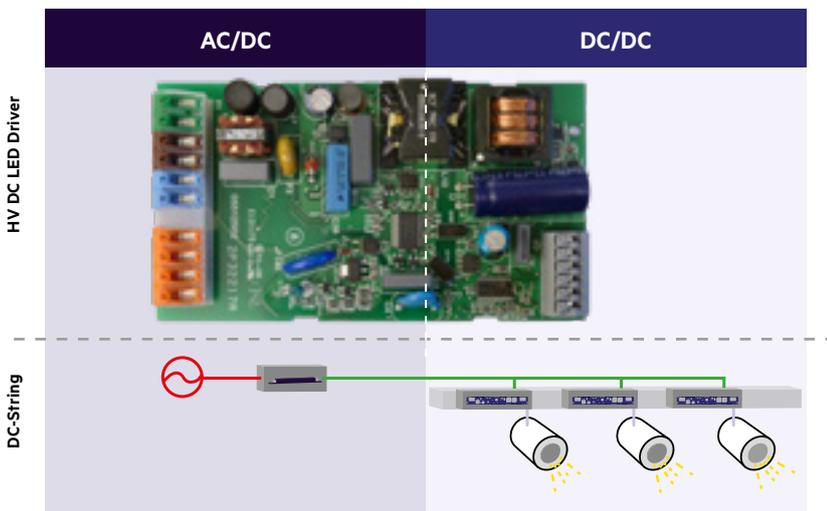
In conventional LED drivers, the AC/DC conversion takes up most of the space. For 48 V DC-String, Tridonic has divided the LED driver into two components. Only the DC/DC LED driver remains part of the luminaire, whereas the AC/DC driver operates independently of the LED modules.
