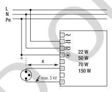
Circuit diagram multiwatt for 22, 50, 70 and 150 W
