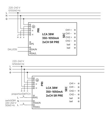
Device with loop through wiring function.
