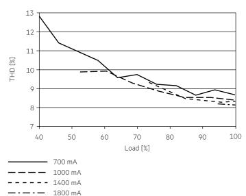
100 % load corresponds to the max. output power (full load) according to the
