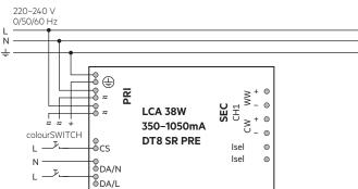
Device with loop through wiring function.
