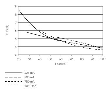
100 % load corresponds to the max. output power (full load) according to the table on page 2.
