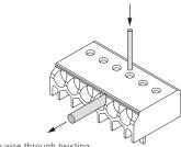
Loosen wire through twisting and pulling or using a  $\emptyset$  1mm release tool
