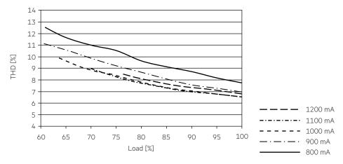
100 % load corresponds to the max. output power (full load) according to the table on page 2.
