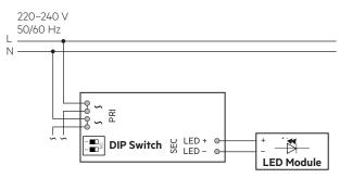
Device with loop through wiring function.
