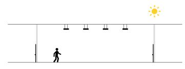
While in daylight mode, the sensor does not activate light when movement is detected.
