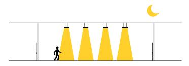
While in night mode, the sensor activates light when movement is detected.
