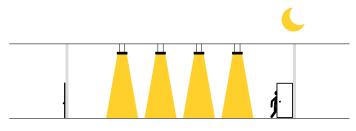
If the moving object leaves the detection area or keeps still, the light will keep on for the duration of the delay time.
