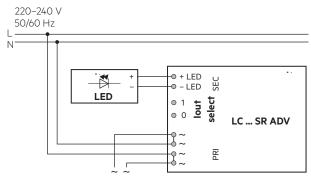
Device with loop through wiring function.
