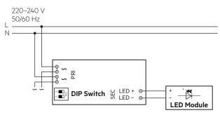
Device with loop through wiring function.
