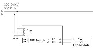
Device with loop through wiring function.
