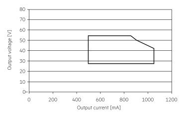
Make sure that the LED driver is operated within the given window under all operating conditions.
