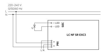
Device with loop through wiring function.
