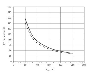
Max. LED current at nominal battery voltageMin. LED current at nominal battery voltage
