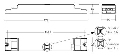
Note: LED driver supplied with duration link in 3 hours position. Remove duration link for 1 hour duration. Duration link must be set before battery and mains connection.
