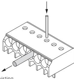
Loosen wire through twisting and pulling or using a  $\varnothing$  1 mm release tool
