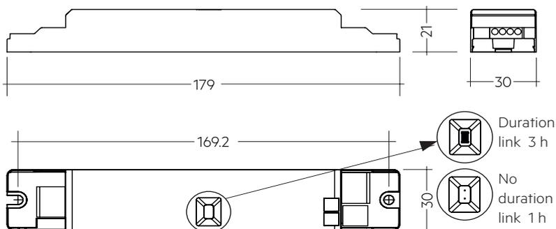
Note: LED driver supplied with duration link in 3 hours position. Remove duration link for 1 hour duration. Duration link must be set before battery and mains connection.
