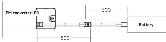
When using an EM converterLED in combination with a NiMH battery, order the CONNECTION CABLE NiMH 500mm separately.
