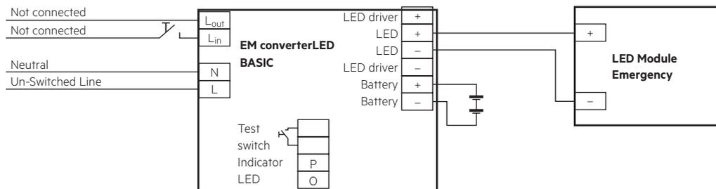
**EM converterLED BASIC with a standard LED driver and one LED module for mains and emergency operation**
