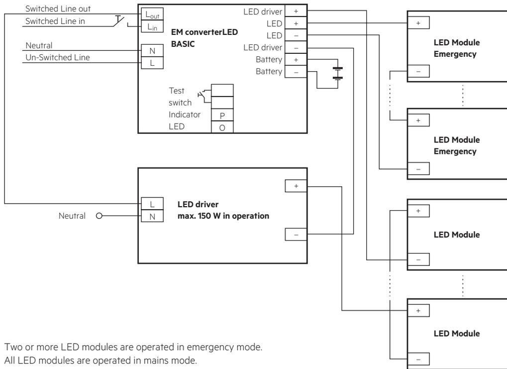
**EM converterLED BASIC with a standard LED driver and parallel operation of LED modules**
