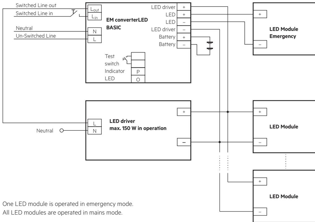
**EM converterLED BASIC with a standard LED driver and parallel operation of LED modules**
