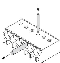
Loosen wire through twisting and pulling or using a Ø 1 mm release tool
