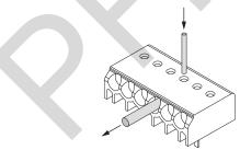
Loosen wire through twisting and pulling or using a Ø 1mm release tool
