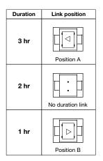
Module supplied with duration link in 3 hours position (position A).
