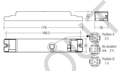
Note: LED Driver supplied with duration link in 3 hours position. Duration link must be set before battery and mains connection. The EM converterLED PRO 135 NiCd is supplied without a duration link.
