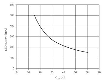
EM converterLED ST 1-9-15 60V UNV Article number: 28002869 NiMH battery, 10.8 V battery voltage 1,410 – 1,720 mA battery discharge current (tolerance)
