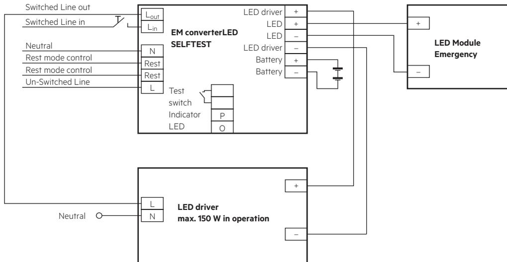
**EM converterLED SELFTEST with a standard LED driver and series operation of LED modules**
