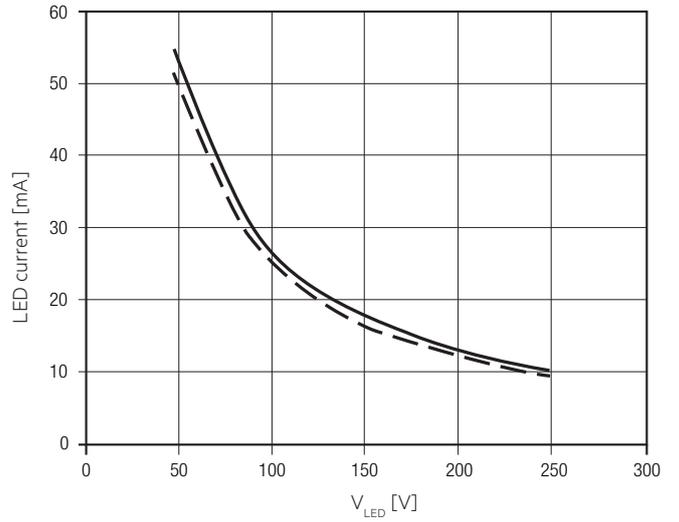
EM converterLED ST 304 LiFePO4 250V
