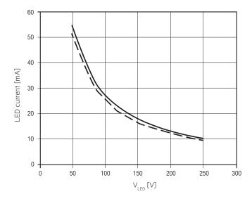
EM converterLED ST 204 MH/LiFePO4 250V Article number: 89800635 NiMH battery, 4.8 V battery voltage 810 – 870 mA battery discharge current (tolerance) LiFePO<sub>4</sub> battery, 3.2 V battery voltage 1,275 – 1,375 mA battery discharge current (tolerance)
