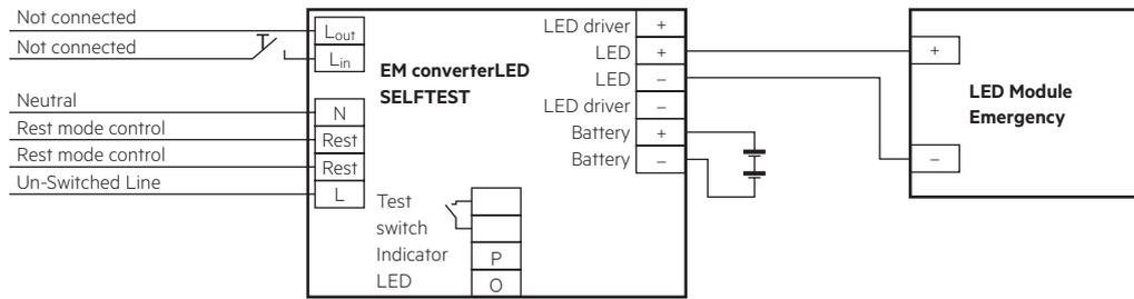
**EM converterLED SELFTEST with a standard LED driver and one LED module for mains and emergency operation**
