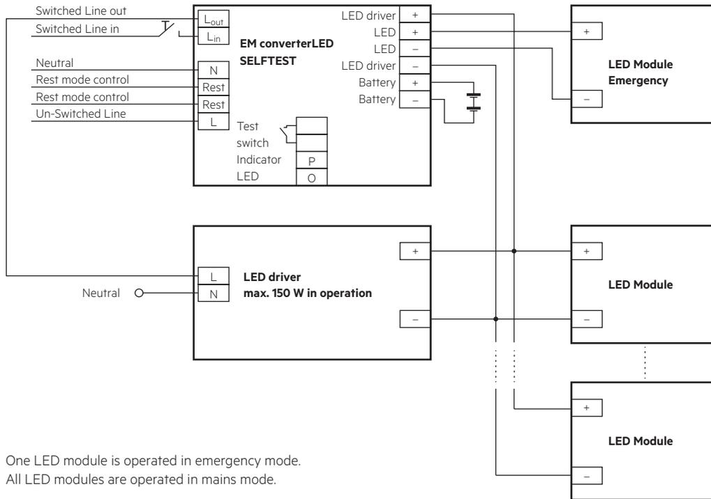
One LED module is operated in emergency mode.
