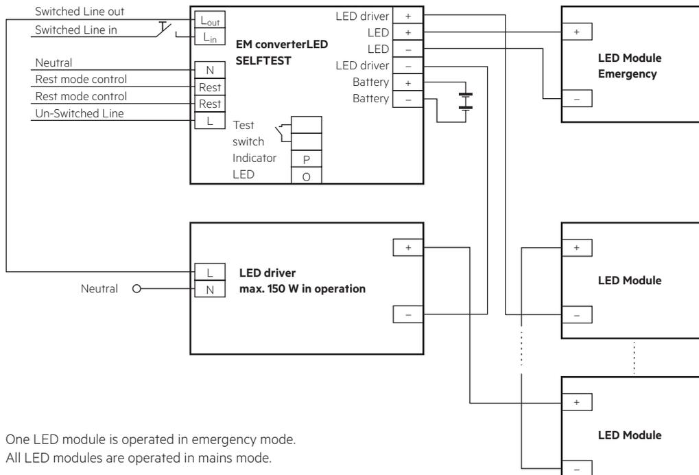
One LED module is operated in emergency mode.
