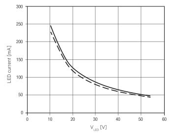
EM converterLED ST 204 NiCd/NiMH 50V Article number: 89800648 4.8 V battery voltage 800 – 860 mA battery discharge current (tolerance)
