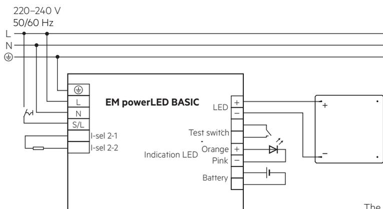
The connected LED module will be used for mains and emergency operation.
