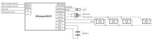
Take care that the LED is connected with the right polarity. LED that are connected to the EM powerLED PRO EZ-3 devices should have a reverse polartity protection device such as a schottky diodes fitted, otherwise irreversible damage could occur if the LED is connected in reverse polarity. Any protection device must be capaple of handling in excess of 1.000 mA.
