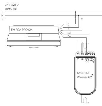
Note: Battery must be connected before mains connection.
