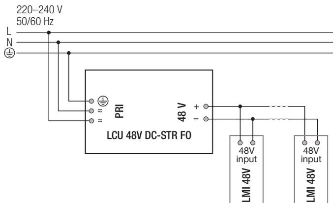
To the LCU 48V DC-STR FO there can be connected eighter LMI 48V fixed output version or LMI 48V dimmable version.
