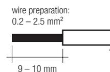
Use one wire for each terminal connector only. Use each strain relief channel for one cable only.
