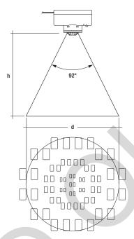
Detection area: 46° Scope: 2.5 m presence detection 5 m motion detection
