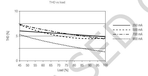
100 % load correspond to the max. output power (full load) according to the table on page 2.
