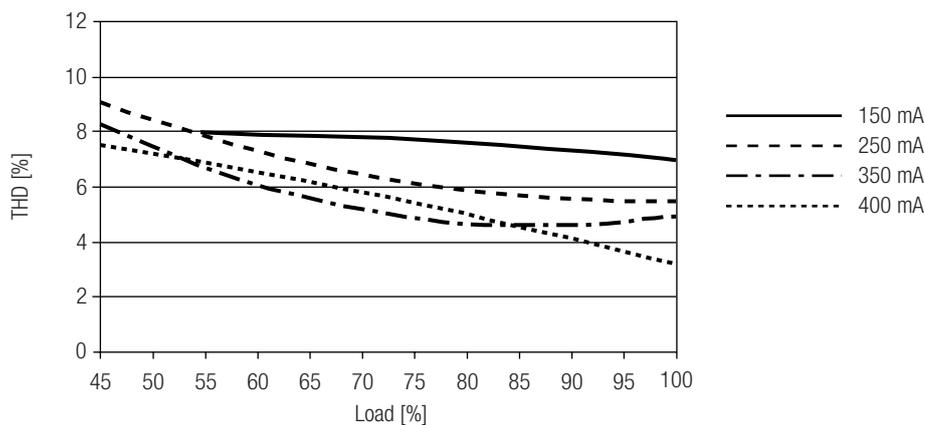
100 % load correspond to the max. output power (full load) according to the table on page 2.
