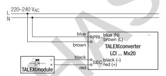
Secondary switching of LEDs is not allowed and may cause damage to the LEDs. The hot plug-in of LEDs during normal operation may result in current peaks of up to 50% above the typical output current.
