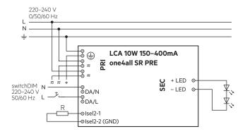
Device with loop through wiring function.
