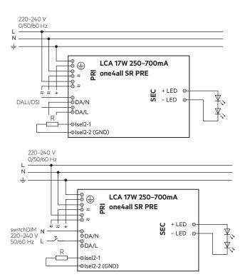
Device with loop through wiring function.
