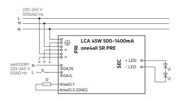
Device with loop through wiring function.
