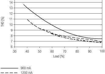
4.4 THD vs load (without harmonic < 5 mA or 0.6 % of the input current)
