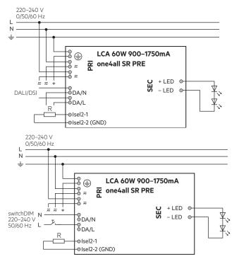
Device with loop through wiring function.
