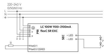
Device with loop through wiring function.
