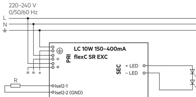
Device with loop through wiring function.
