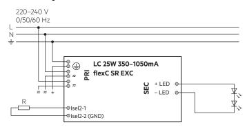
Device with loop through wiring function.
