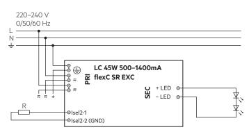
Device with loop through wiring function.
