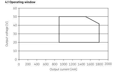
Make sure that the LED driver is operated within the given window under all operating conditions. Coming below the specified minimum output voltage of the LED driver may cause the device to shut-down.
