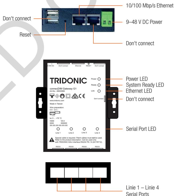
**!** Reset button will trigger a reboot of the Gateway. Data stored on the Gateway will not be deleted.
