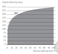
Dimming characteristics as seen by the human eye and is based on the DSI curve.
