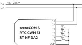
For wiring use stranded wire with ferrules or solid wire from 0.2 to  $1.5 \text{ mm}^2$ . Maximum cable length between momentary switch and sceneCOM S is 50 cm.
