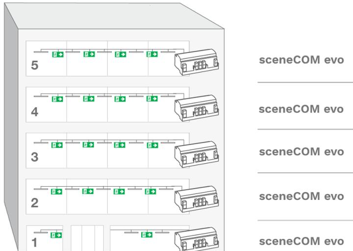
The *sceneCOM* web application provides the option of using just one *sceneCOM evo* control device to automate up to 192 self-contained emergency luminaires. It is therefore suitable for small buildings or individual floors, as shown in the figure on the left.
