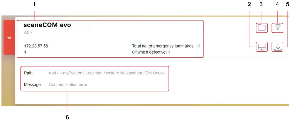
Figure 3: Details about monitoring the functionality of self-contained emergency luminaires
