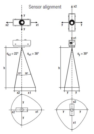
The diameter of the detection area depends on the detection angle of the sensor and the height at which it is mounted.
