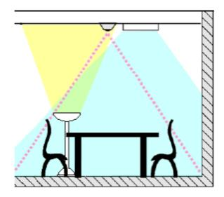
Position the sensor so that it is not directly exposed to other artificial light sources (e.g. free-standing luminaires in the room).
