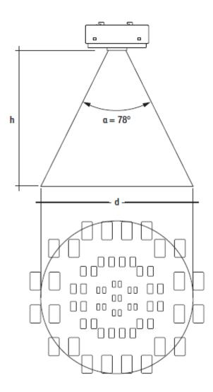
The diameter of the detection area depends on the detection angle of the sensor and the height at which it is mounted. The mounting height also has an effect on the sensor's accuracy. The position and mounting height produce two different detection areas:
