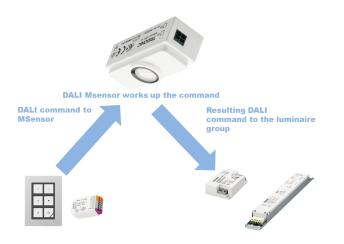
Like DALI control gear, the DALI MSensor reacts to commands that are sent to it, i.e. commands sent to its DALI address, DALI group (luminaire group), or to broadcast commands.
