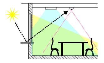
\_ Position the sensor so that it is not directly exposed to sunlight:
