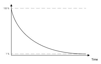
The dimming range is controlled by adjusting the amplitude of the current. The current value specified for the device corresponds to a dimming level of 100 %. The amplitude of the current is reduced to reduce the dimming level. The logarithmic dimming curve is stepless and adapted to the human eye.
