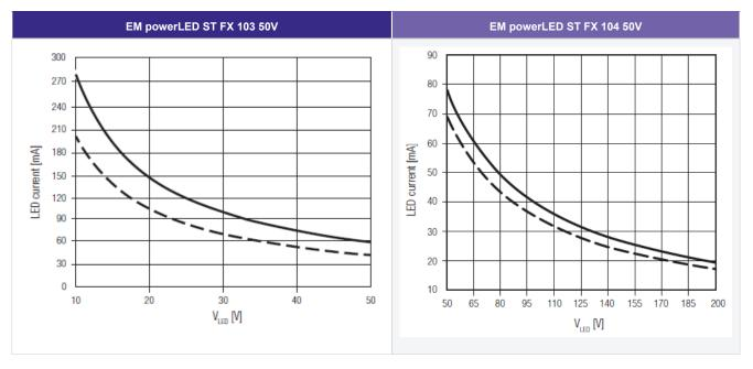
Knowing the total forward voltage of all LED modules, the value for the LED current can be read from the current/voltage curve:
