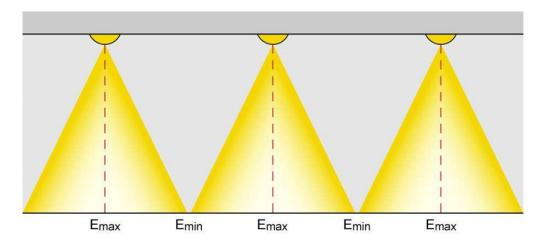
Fig.: Example of lighting for an escape route ( $E_{max}$ :  $E_{min}$  =< 40:1 lx)
