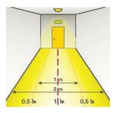
Fig.: Example of horizontal illumination of escape routes
