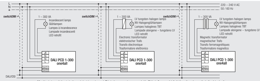
**UK** Digital leading-edge or trailing-edge phase control dimmer for dimming LV tungsten-halogen lamps in conjunction with electronic transformers or magnetic transformers and ohmic light sources with a total connected load of 1-300 VA. The digital phase dimmer is compatible with LED retrofit lamps or LV halogen LED retrofit lamps that are operated by an electronic or magnetic transformer.
