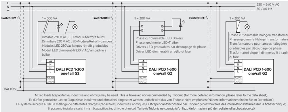
**UK** Digital leading-edge or trailing-edge phase control dimmer with one4all interface to control dimmable LED retrofit bulbs, phase cut dimmable LED drivers and dimmable halogen transformers with a total power of 1 to 300 VA.
